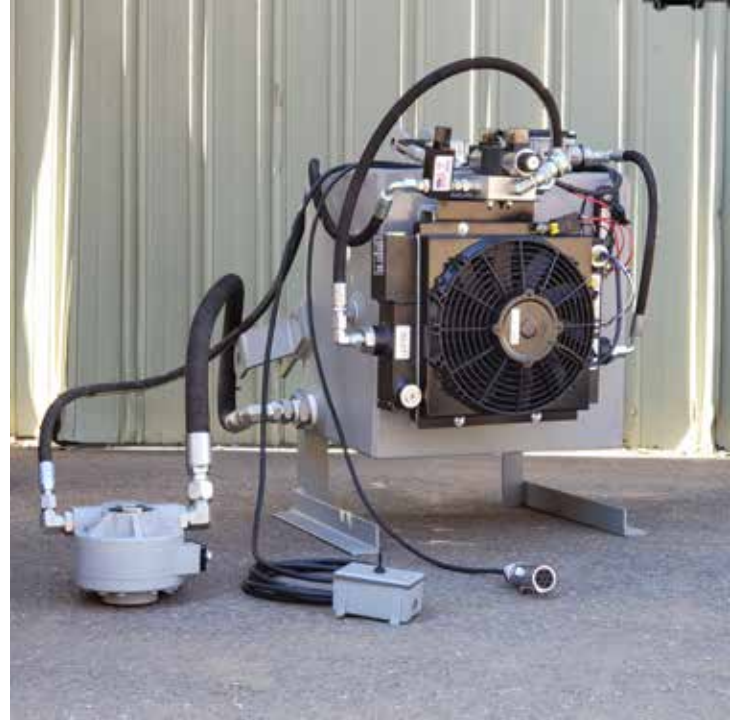
Hydraulic Power Pack 3-Point Mounted, PTO Driven, Electric over Hydraulic Forward/Reverse Controls, Temperature Activated Cooling
