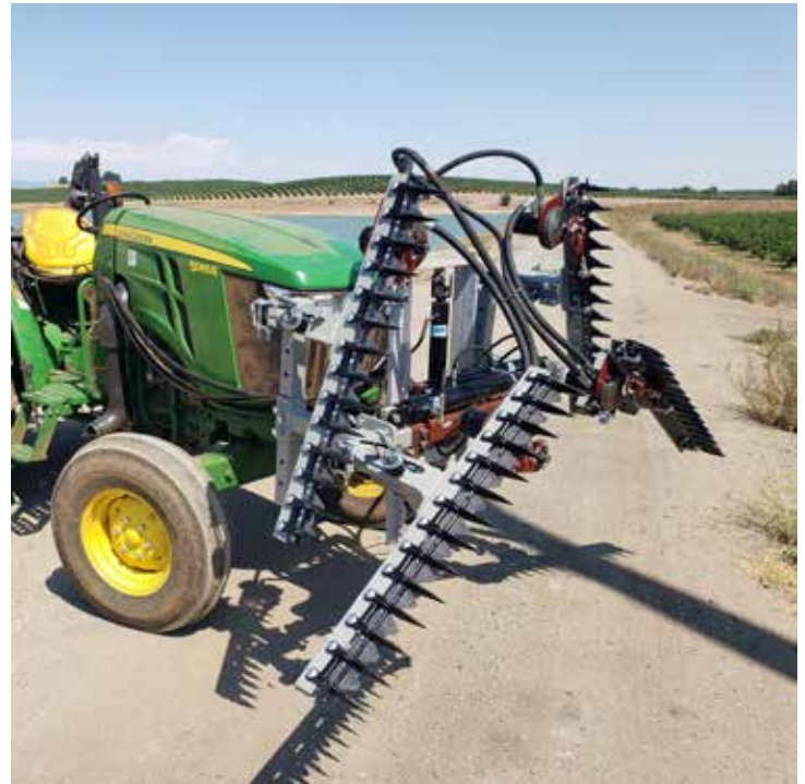
SD Frame, Standard Hydraulic Width, Quad 3.5' Single Sickle Bar Trimmers, Arranged for Hedging/Skirting
