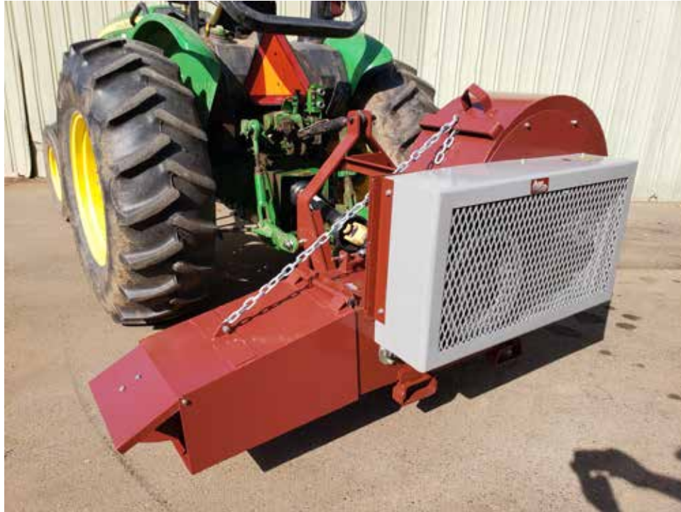
Single Berm Blower Category 2 3-Point Mounting, 540 RPM PTO driven 13,000 CFM Easy-transport folding nozzle
