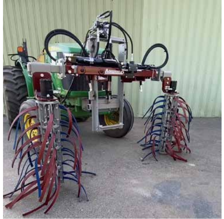
SD Frame, Standard Hydraulic Width, Suckering/Thinning Arms, 4-Segment Suckering Heads with Belts
