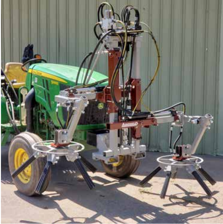
Terracing Frame, Narrow, Individual Left/Right Motor Control, Poly Rod Sweeper Heads on Breakaway Arms
