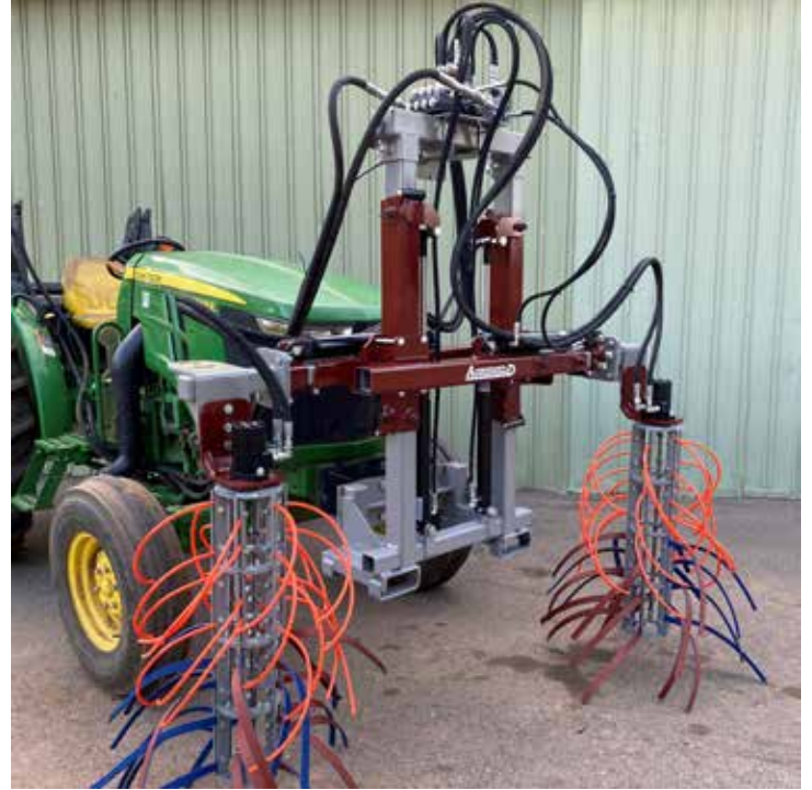
Terracing Frame, Wide, Suckering/Thinning Arms, 4-Segment Suckering Heads with half whips/half belts
