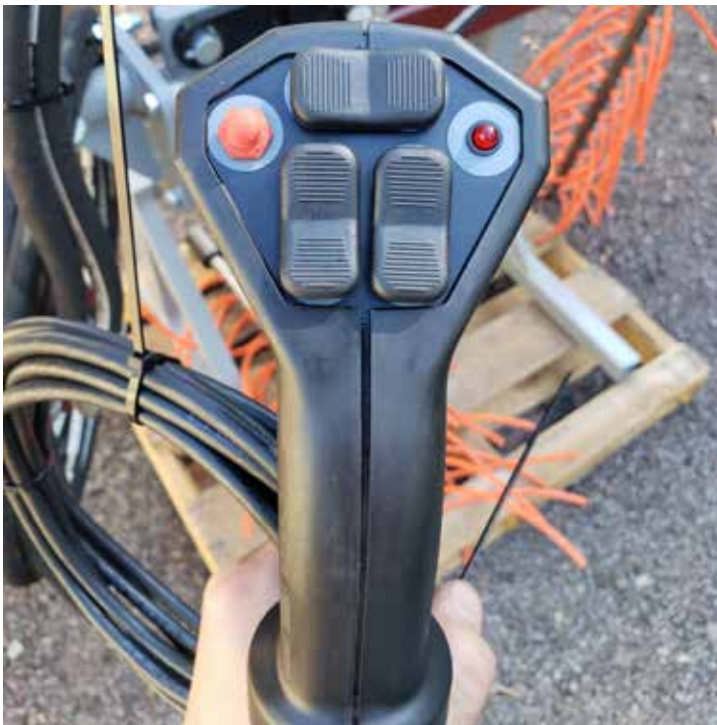
Electronic Controls option for Implements Left/Right Height Cylinder Control, In/Out Cylinder Control, Motors On/Off Button, LED Motor Status Indicator
