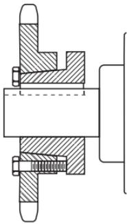
1. Be sure the tapered cone surfaces of the bushing and the inside of the driven product are clean and free of anti-seize lubricants.
