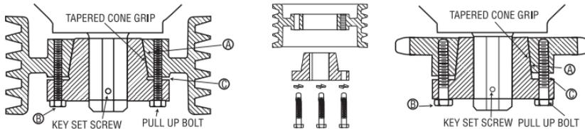
1. Be sure the tapered cone surfaces of the bushing and the inside of the driven product are clean and free of anti-seize lubricants.
