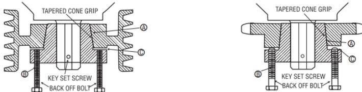
1. Remove pull-up bolts and screw them into TAPPED holes in bushing flange and against hub of sheave or sprocket to break cone grip.
